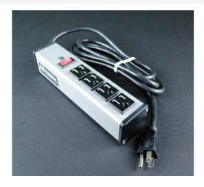
Four outlets, rugged gray aluminum housing, 15A, lighted switch. 6' (1.8m) 14/3 SJT black cord with NEMA5-15 plug. Length 9 1/4" (235mm). Receptacle center-to-center 1 1/4" (32mm). Snap-on, slide-off mounting.
