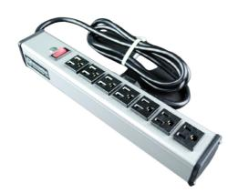
Seven outlets, rugged gray aluminum housing, 15A, lighted switch. 15' (4.6m) 14/3 SJT black cord with NEMA5-15 plug. Length 13'' (330mm). Receptacle center-to-center 1 1/4'' (32mm). Snap-on, slide-off mounting.
