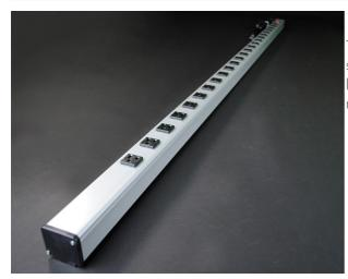
Twenty-four outlets, rugged gray aluminum housing, 15A, lighted switch, 6' (1.8m) 14/3 SJT black cord with NEMA5-15 plug. Length 72'' (1.8m). Receptacle center-to-center 2 1/2'' (64mm). Snap-on, slide-off mounting.
