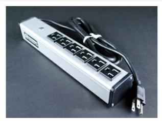
Six outlets, rugged gray aluminum housing, 15A. 6' (1.8m) 14/3 SJT black cord with NEMA5-15 plug. Length 12 1/4" (311mm). Receptacle center-to-center 1 1/4" (32mm). Snap-on, slide-off mounting.
