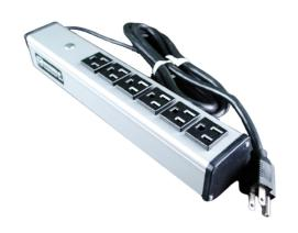
Six outlets, rugged gray aluminum housing, 15A. 15' (4.6m) 14/3 SJT black cord with NEMA5-15 plug. Length 12 1/4'' (311mm). Receptacle center-to-center 1 1/4'' (32mm). Snap-on, slide-off mounting.
