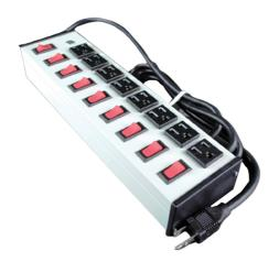
Eight individually switched outlets, lighted on/off switch, putty white finish aluminum housing, 15A. 15' (4.6m) 14/3 SJT black cord with NEMA5-15 plug. Length 13'' (330mm), width 3 1/2'' (89mm). Receptacle center-to-center 1 5/16'' (33mm). Snap-on, slide-off mounting.
