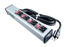
Four individually switched outlets, lighted on/off switch, rugged gray aluminum housing, 15A. 15' (4.6m) 14/3 SJT black cord with NEMA5-15 plug. Length 13" (330mm), width 2" (51mm). Receptacle center-tocenter 2 1/8" (54mm). Snap-on, slide-off mounting.
