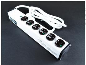
Six outlets. Rugged white aluminum housing. 6' (1.8m) 14/3 SJT white cord with NEMA5-15 plug. Length 13 1/4" (337mm). Receptacle center-to-center 1 1/2" (38mm). Snap-on, slide-off mounting. Not for use in critical care enviornments. NOTE: Not for use where Article 517 of NEC requires Hospital Grade Outlets.
