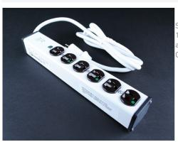
Six outlets. Rugged white aluminum housing. 15' (4.6m) 14/3 SJT white cord with NEMA5-15 plug. Length 13 1/4'' (337mm). Receptacle center-to-center 1 1/2'' (38mm). Snap-on, slide-off mounting. cTUVus Listed as Medical Electrical Equipment. NOTE: Suitable for use where Article 517 of NEC requires Hospital Grade Outlets.
