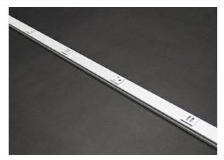
Available in 5' (1.5m) length with 9" spacing. 15A tamper-resistant receptacles. 3-wire, #12 THHN (1 hot, 1 neutral and insulated ground conductor). .040" (1.0 mm) steel housing. Packed two per carton. Each unit supplied with one (1) Coupling and two (2) Blank End Fittings. USB is 2.4 Amps (shared between two ports) 5VDC. Please note the charging load on one module will not affect the charging performance of the other USB modules in the product.
