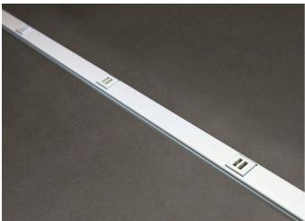
3' (914mm) length with 12" spacing. USB is 2.4 Amps (shared between two ports) 5VDC. .040" (1.0mm) steel housing. Packed two per carton. Each unit supplied with one (1) Coupling and two (2) Blank End Fittings. Each USB module provides 2 ports with 2.4 Amps of shared charging. Please note the charging load on one module will not affect the charging performance of the other USB modules in the product.
