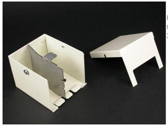
Feeds 2400D Series Raceway. Back has two 1/2'' trade size KOs and two rectangular KOs for communication cabling. Additional 1'' and 3/4'' concentric trade size KOs on each side.
