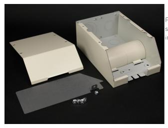
Feeds 2400 and 2400D Series Raceway. Has 1/2'', 3/4'', and 1'' trade size KOs on back and end. Removable divider and radiused insert included.
