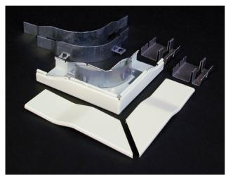
90 degree flat elbow with integral dividers. Provides 2" (51mm) full capacity cable bend radius control for fiber optic and UTP/STP cable installations. Ideal for lay-in or pull-through installations. Two couplings included.
