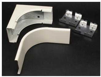
90 degree internal corner elbow provides 2'' (51mm) cable bend radius control for fiber optic and UTP/STP cable installations. Two couplings included.
