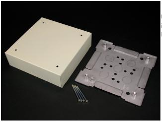
Used as a tee, cross, junction box, or for branch circuit extensions in 3000 Series Raceway. Cover has raceway twistouts on all sides. Base has five 1/2" trade size KOs and four fixture mounting holes.
