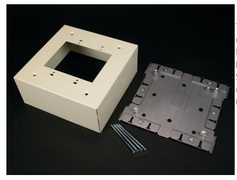
Two-gang. For standard 30A, 50A, and 60A receptacles. Four sides of cover have one set of combination twistouts for 3000 Series Raceway. Hole cut in cover: 3 3/4'' x 2 7/8'' (95mm x 73mm). Base has five 1/2'' trade size KOs. NOTE: Certified to Canadian Safety Standards for sale in Canada. When ordering these products, change the ''V'' color prefix to ''CV'' or the ''G'' color prefix to ''CG'' to denote the Canadian versions.
