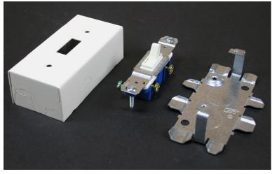
Single pole switch included. Accepts standard singlegang switches including three-way. Cover has twistouts for 500 or 700 Series Raceway on each end and sides. Twistouts on ends of box permit running raceway close to interior trim. Base has 1/2" trade size KOs. NOTE: Certified to Canadian Safety Standards for sale in Canada. When ordering these products, change the "V" color prefix to "VC" to denote the Canadian versions.
