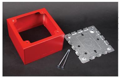
For surface mounting of alarm devices and safety signals designed to fit into 4'' (102mm) square back boxes. Available in red and ivory finishes. Cover is 2 3/4'' (70mm) deep and has three twistouts for raceways on each side. Base has 1/2'' and 1'' concentric and single-gang box KOs. Accepts NEMA double-gang standard faceplates.
