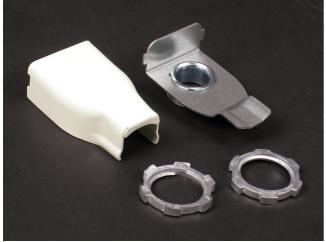
Connects raceway at right angles to conduit boxes or panel boxes that have 1/2" trade size conduit KOs. When used with 700 Series Raceway, break out crescent twistout in cover.
