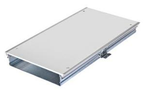
Used to change direction of Trenchduct run 45° in either direction. Length, width, and depth determined by the catalog number. Use partition to separate services (ordered separately for standard product).
