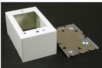
For deep devices such as momentary contact, remote control switches, and hospital signaling system devices. Base has 1/2" trade size KOs. Larger gang boxes available by special order. Single-gang: 4 5/8" L x 2 7/8" W (117mm x 73mm). Accepts NEMA single-gang standard faceplates. NOTE: Certified to Canadian Safety Standards for sale in Canada. When ordering these products, change the "V" color prefix to "vc" or the "WH" color suffix to "WHC" to denote the Canadian versions.
