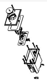
Includes single-gang box, device plate with two openings for communication devices, and brass cover with one screw plug. For hole cut dimensions, see installation instructions sheet. Box Dimensions: 2 1/8" W x 3 3/4" L x 3 7/8" D (54mm W x 95mm L x 98mm D) Device Plate: 3 1/8" W x 4 15/16" L (79mm W x 125mm L).
