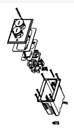
Includes single-gang box, 106 adapter with four openings for communication devices, and brass cover with two screw plugs. For hole cut dimensions, see installation instructions sheet. Box Dimensions: 2 1/8" W x 3 3/4" L x 3 7/8" D (54mm W x 95mm L x 98mm D) Device Plate: 3 1/8" W x 4 15/16" L (79mm W x 125mm L).
