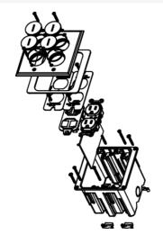
Includes dual-gang box, one 15A tamper-resistant duplex receptacle, 106 adapter with four openings for communication devices, and brass cover with four screw plugs. For hole cut dimensions, see installation instructions sheet. Box Dimensions: 3 1/4" W x 3 3/4" L x 3 7/8" D (83mm W x 95mm L x 98mm D) Device Plate: 4 7/8" W x 5 1/16" L (124mm W x 129mm L).
