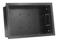
The WMPAC525F and WMPAC526F simplify flat panel installation by providing an organized, recessed space for routing excess cables and for attaching surge protectors/power conditioners. The addition of the flange adds an aesthetic trimmed appearance and drywall mounting capability.
