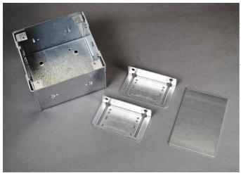
Slide-in dividers separate the box for power and communication services. Adjustable mounting brackets offer flexibility to flush mount box in 1/2", 5/8", 1", and 1 1/4" (12.7mm, 15.9mm, 25mm, and 32mm) wall thicknesses. Ordering Data: 4 3/4" L x 5" W x 3 1/4" D (121mm L x 127mm W x 83mm D), 2-Gang, 1/2", 3/4", and 1" trade size KOs. NOTE: Certified to Canadian Safety Standards, for sale in Canada. When ordering, add "C" suffix to part number to denote the Canadian version, i.e., "WSB42-2C".
