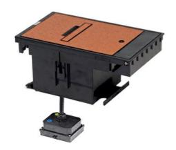
The brown Outdoor Ground Box cover assembly is prewired on a single circuit with (2) 20A weather resistant duplex receptacles. CAUTION: All ground box electrical circuits must be protected by a Ground Fault Circuit Interrupter upstream from the ground box.NOTE: Cover must be closed while in use. Use only molded plug and cord assemblies that are rated for outdoor use.NOTE: Maximum length of plug allowed at end of cord is 3" [76mm].
