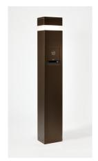
Outdoor charging station with an LED area light to enable device charging during the day and after dark. Area light ensures the station stands out from standard bollards and clearly indicates charging. Station includes one 4-Port USB-A outlet and two duplex 20A, weather-resistant GFCI Receptacles with USB-C.
