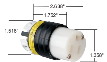
Dimensions for 15 & 20 Amp GCM Straight Blade Connector
