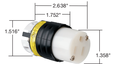
Dimensions for 15 & 20 Amp GCM Straight Blade Connector
