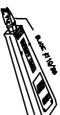
REQUIRED TERMINATION TOOL OR EQUIVALENT (TUL) OR HOOPER (TUL) TERMINATION OF CABLE PAIRS
